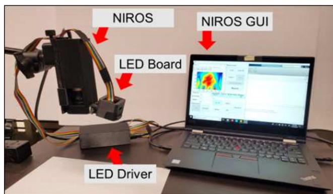
Fig. 6 : Near Infrared Optical Scanner (NIROS) operated using a laptop and stabilized using an articulating arm.
