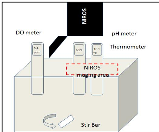
Fig. 4. Experimental set-up of phantom studies (including scatterers, via 45% whole milk in water). Imaging performed by NIROS, along with Dissolved Oxygen (DO) meter, pH meter, and thermometer.
