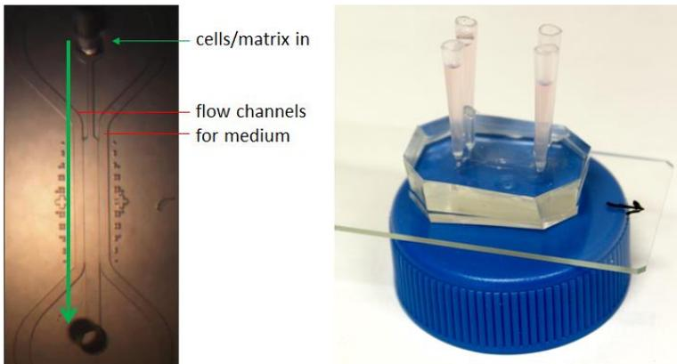
**Fig. 1C:** Implementation of phase guide device for static culture.
