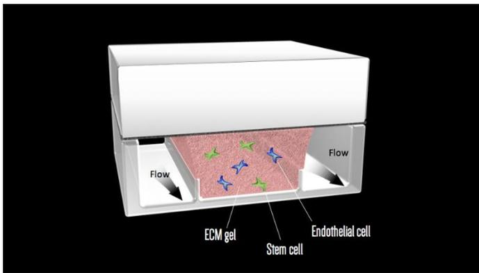
**Fig. 1A:** Conceptual design of phase guide device filled with cells and ECM.
