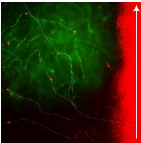
**Fig. 2C:** Anastomosis and perfusability of the capillaries illustrated by flowing fluorescent microbeads through the vascular network from one flow channel to the other.
